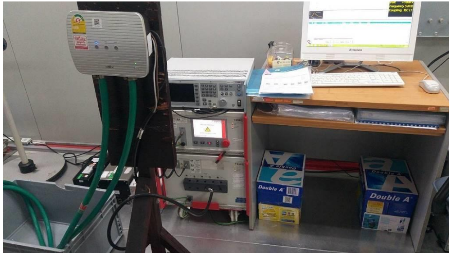
Electrical Fast Transient / Burst Immunity Test Setup
