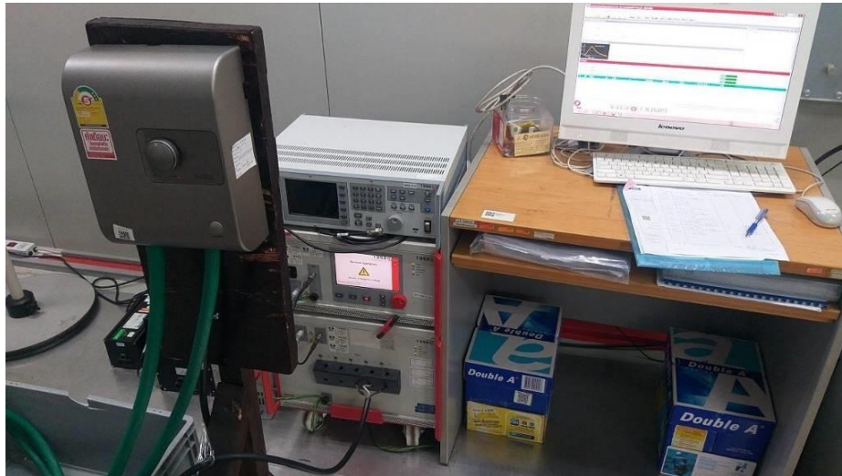
Voltage Surge Immunity Test Setup
