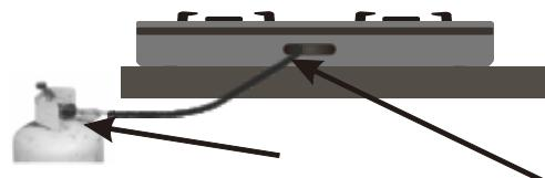
5. If growing bubble appear, there ia a leak. Turn off the gas supply in event of gas leak. It leaks cannot be stopped, do not try to repair. Replace a new one.
